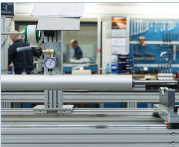
Concentricity tested with an accuracy to a hundredth.
