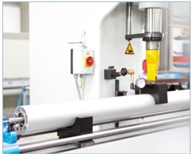
Precision straightening of technical rollers.
